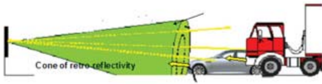
Traffic Sign: Cone of reflectivity: efficient return and distribution of light emitted by vehicles.
