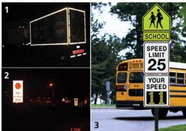
1) Vehicle Conspicuity Markings in S. Africa: do you see the second truck? 2) Recommended signage (night vision) 3) Special fluorescent colours and driver feedback signs
